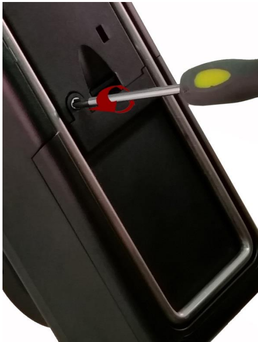
Step 1 - Remove security screw with Phillips screwdriver.
